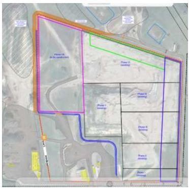
The orange outline is a ring-road that will provide access around the landfill for equipment access or emergencies. The final phase of the landfill will require the existing scale house and garage to be relocated outside of the useable airspace. Again this is likely in the 10-15 year range, but it is unfortunate that permanent structures were built where they were.
