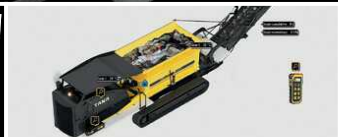
A real time view to the machine through TANA ProTrack® opening a quick and accurate trouble-shooting and possibilities for preventative maintenance by TANA Service Center.
